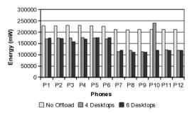
Figure 3: Comparison of application energy usage
